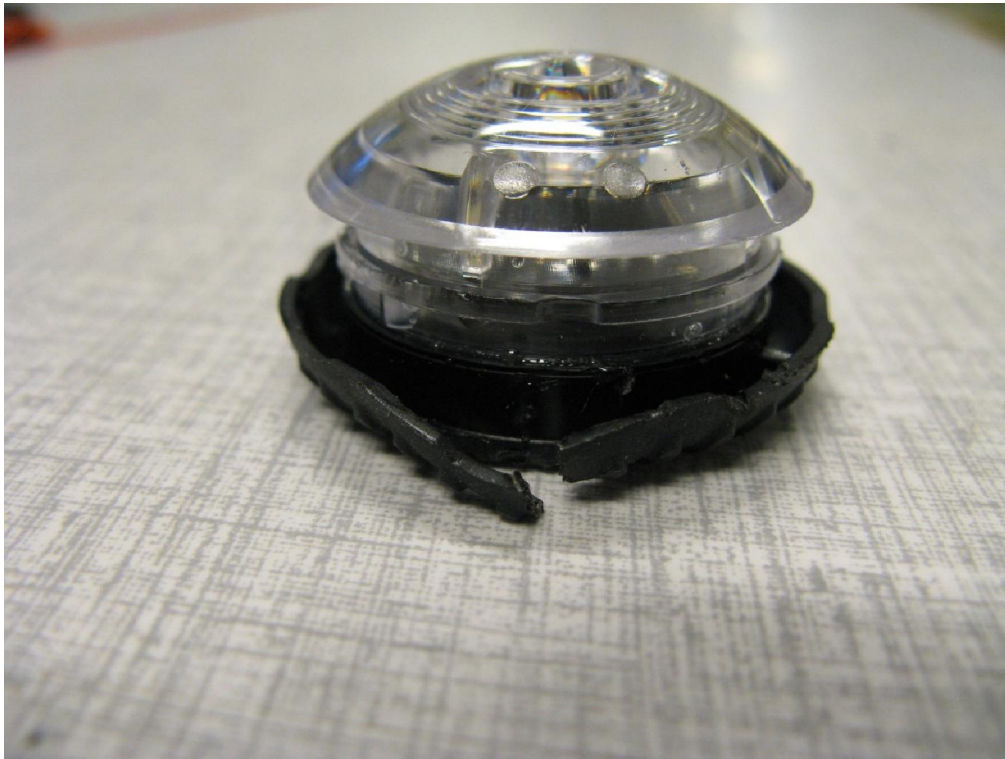
Picture 8: EUT after the IPX8-test; no ingress of water.
