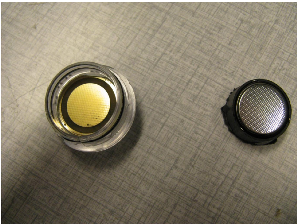
Picture 9: EUT after the IPX8-test; no ingress of water.
